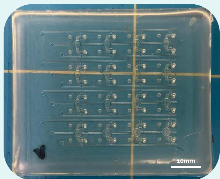
Final PDMS microfluidic device with 16 integrated peristaltic pumps, made with 2mm x 1mm x 200µm macro-valves.
